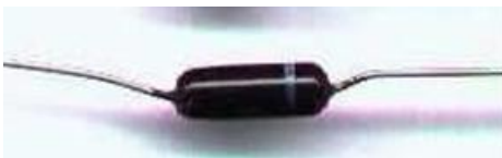
A diode with a stripe that marks the negative cathode. So you know how to switch it in a circuit. (source: Wikipedia public domain)
