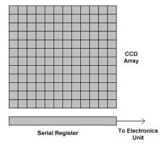
Figure 11: a 12x12 photosite CCD
