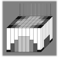
When a photon hits a square, an electron is released. The electrons are stored within the walls of a photosites.
