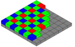
Figure 13: the colour-filtering mask on a CCD (source: wikipedia)
