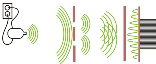
Figure 2 Quantum Theory assumes that a field is connected to particles like an electron. The waves of that field pass through the slits and interfere (constructively and destructively) in different places. Where the amplitudes are large there is a large chance that a discrete and local energy packet is given off by the field. That is what we observe as a particle.
