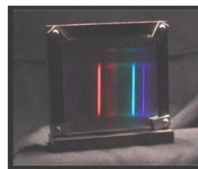
Figure 12 The characteristic line spectrum of atomic hydrogen is composed out of 3 sharp lines: a red, a blue and a violet line.
