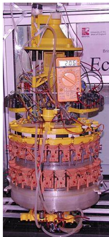
Figure 2. EcoBot III, MFC-based autonomous robot (source: Wikipedia)
