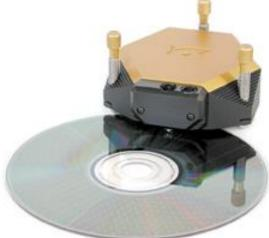
Figure 2: AFM measurements of a compact disc. The estimated time to get the 3-dimensional picture is 10 minutes.
